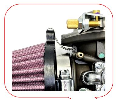
Fit the safety wire between the carburettor and the filter . Use the enclosed aviation safety thread. Connect the wire as indicated between the carburettor and the filter slot using special pliers p/n: 00230P or p/n: 00230G see figure below.
